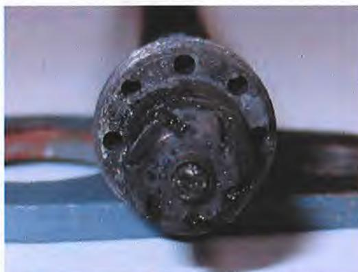
Figure 11. View of the bed material and the humins injection probe tip after the combustion test with humins.
