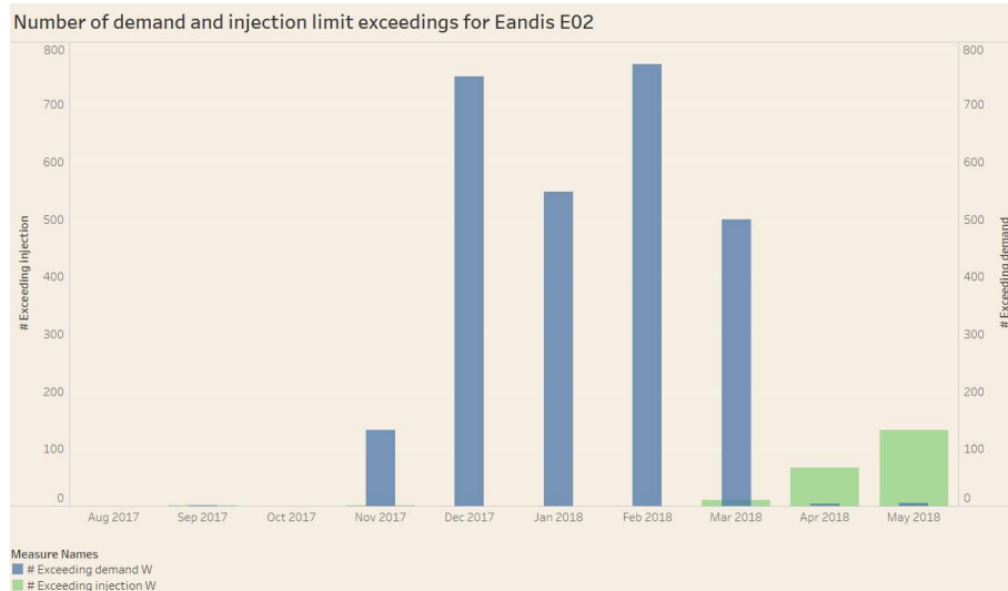
Figure 17 Eandis_E02 exceedings with HEMS installed
