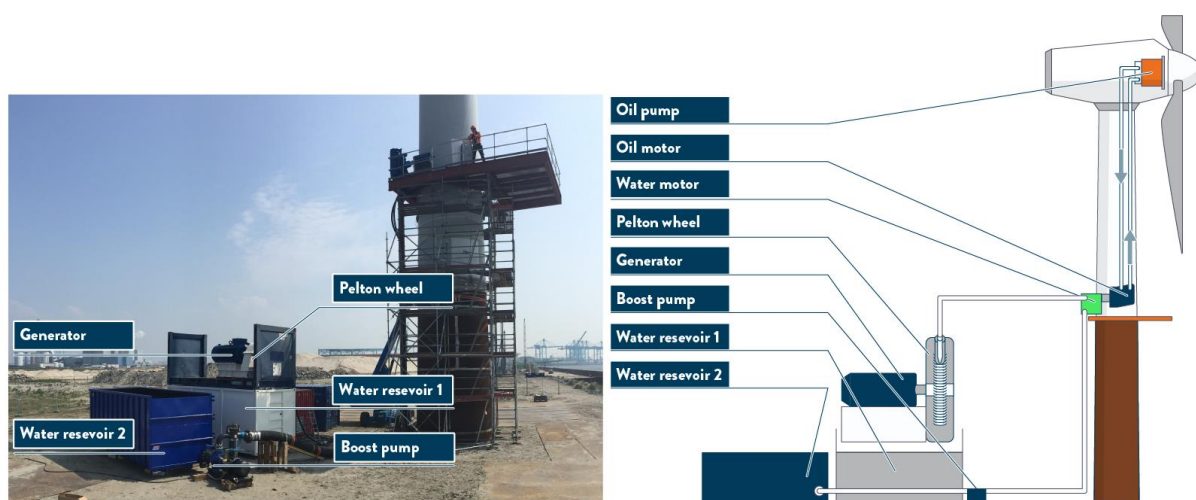
FIGURE 1 | OVERVIEW OF ONSHORE TEST SET-UP
