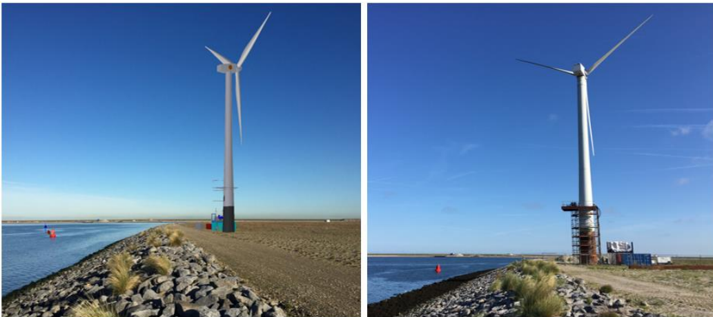
FIGURE 2 | COMPARISON BETWEEN DESIGN (LEFT: 3D RENDER) AND ACTUAL TEST SET-UP (RIGHT: PHOTO OF FINAL SET-UP)
