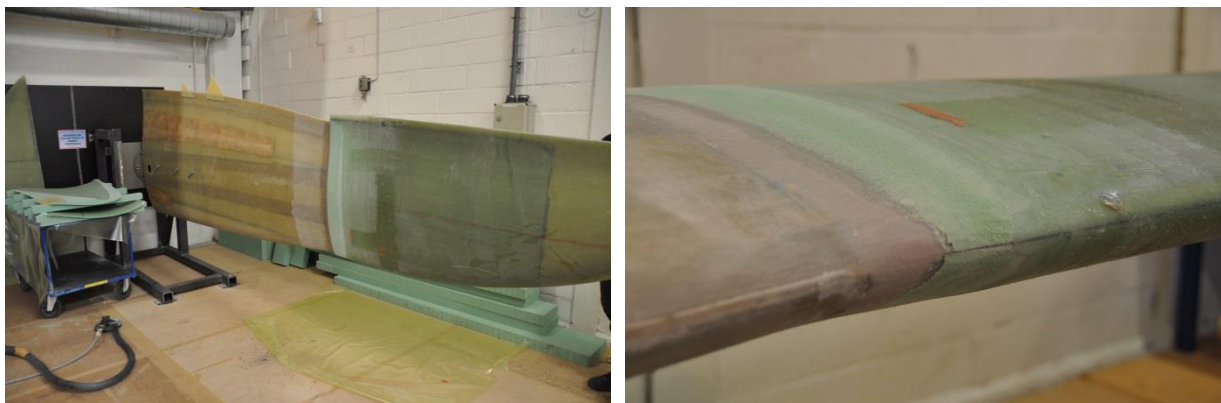
Figure 5-12: Glued tip pre- and post-grinding
