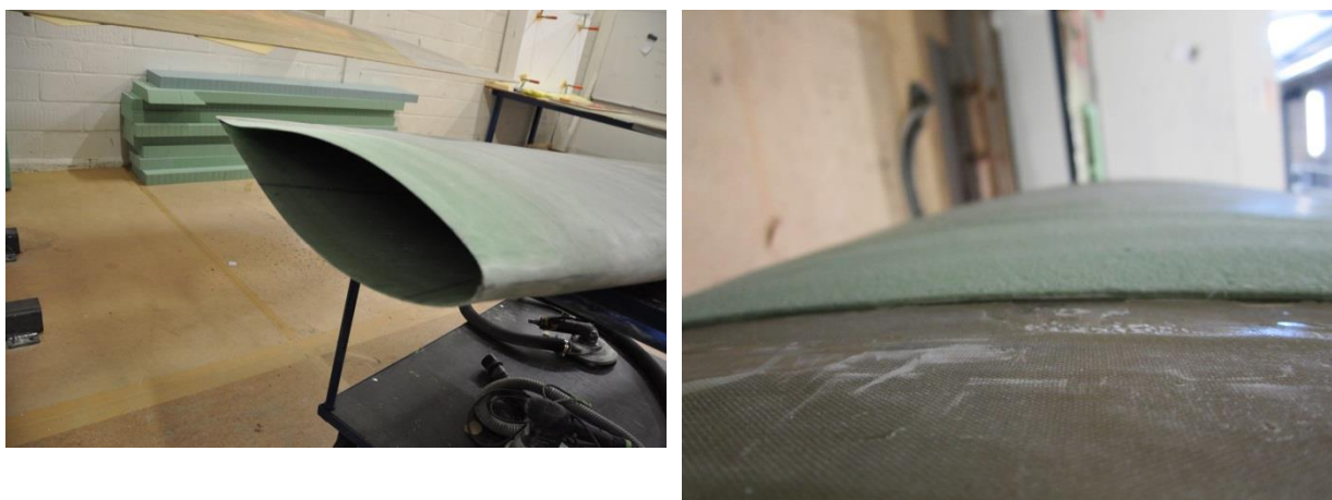
Figure 5-6: Grinded prototype tip for smooth transition
