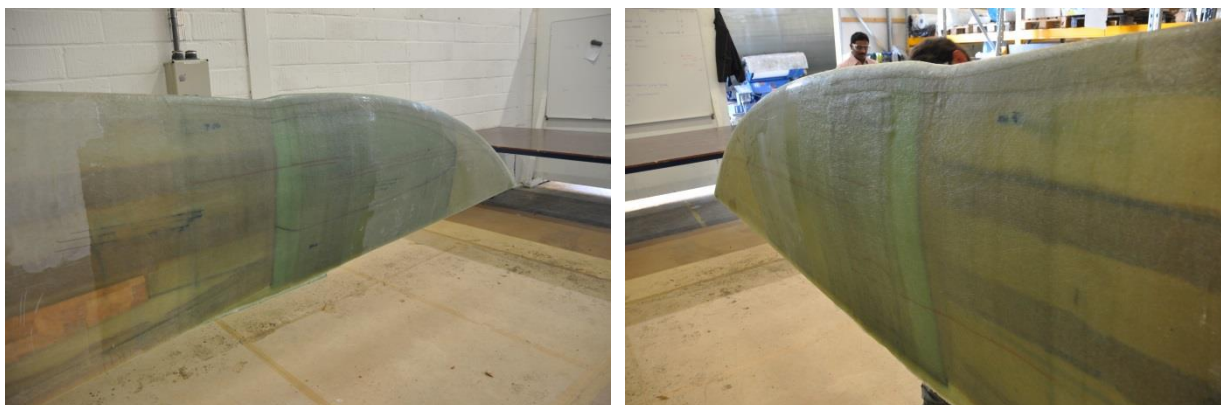
Figure 5-13: Connection after over-lamination process has finalized
