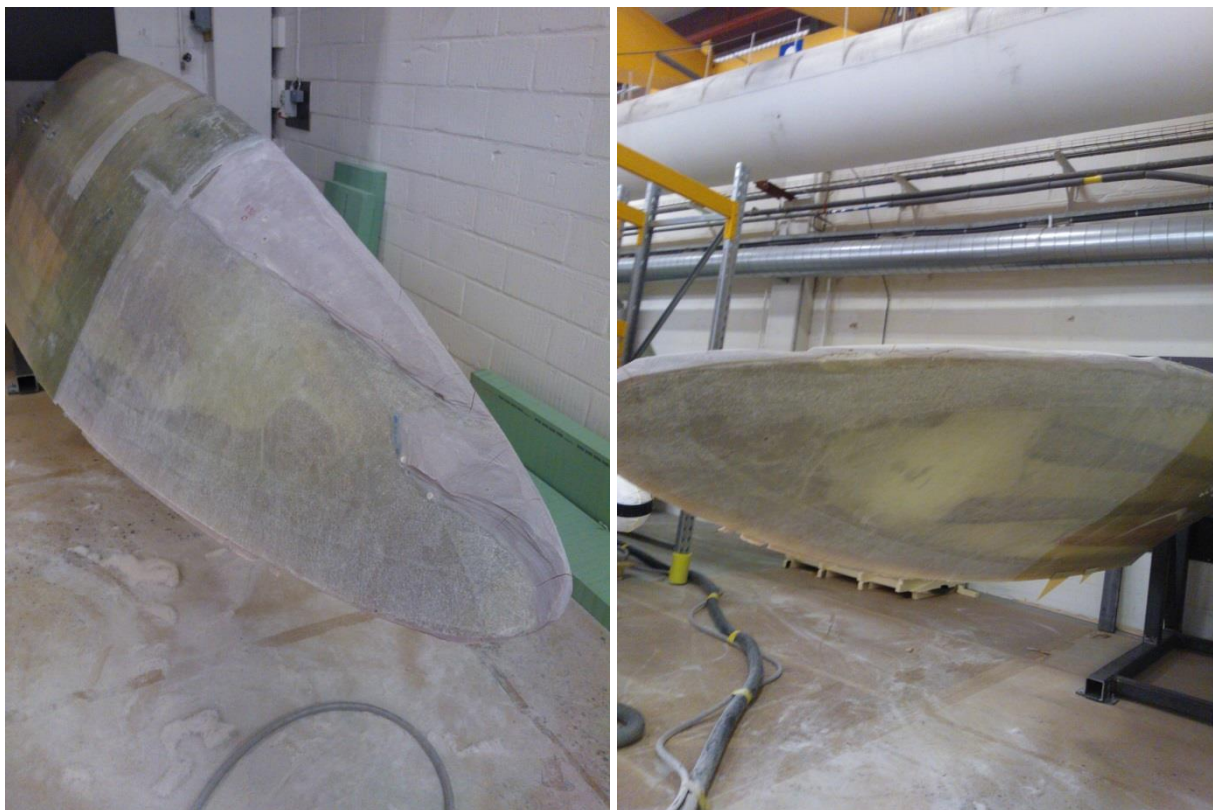
Figure 5-22: partially grinded LM38.8P surface (left) and fully grinded LM38.8P surface (right) after removal of prototype extension
