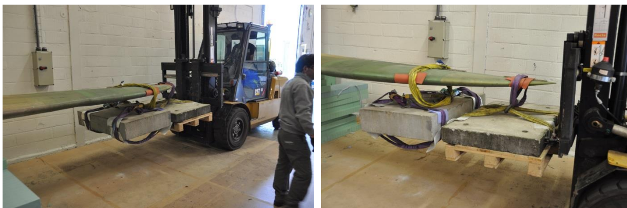
Figure 5-17: Static Extreme load test – Flapwise direction
