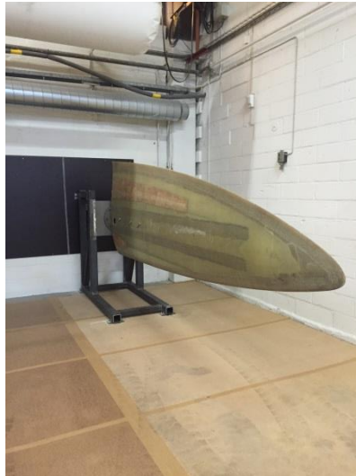
Figure 5-2: LM38.8P tip mounted on rotatable support used for manufacturing and testing
