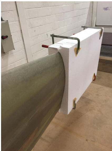
Figure 5-3: Styrofoam negative – checking the internal geometry
