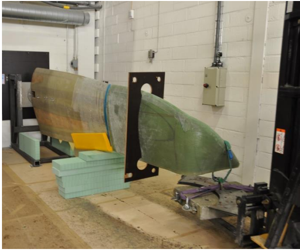
Figure 5-19: Static Extreme load test Winglet - Edgewise direction
