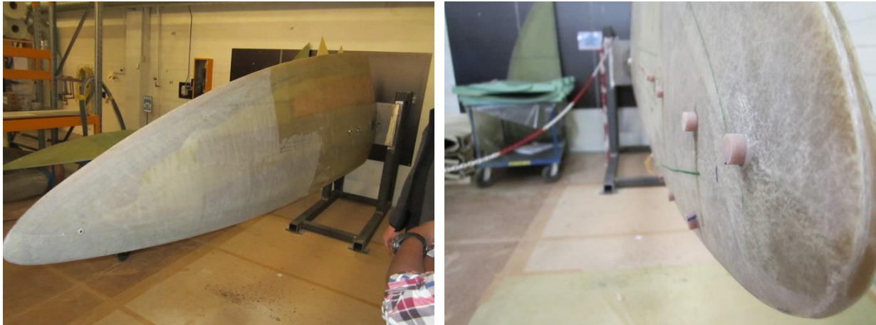
Figure 5-8: Grinded LM38.8P surface and installed distance plugs
