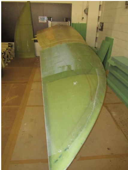
Figure 5-5: Prototype Conventional Tip slid over LM38.8P Tip
