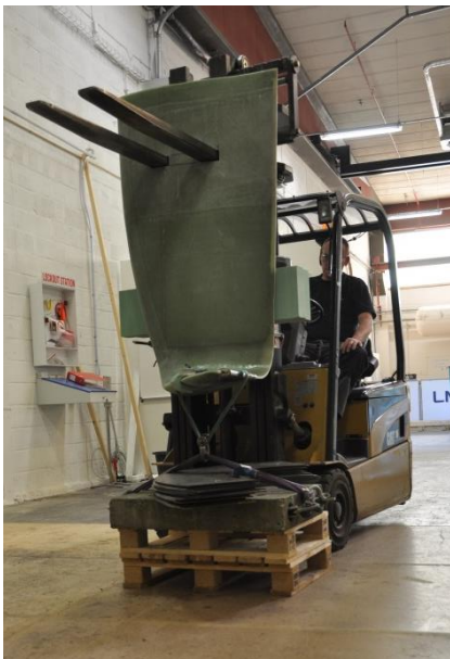
Figure 5-20: Static Extreme load test Winglet – Flapwise direction
