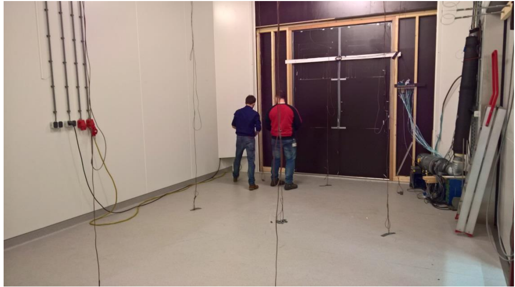
Figure 4: The cold room with a view of the wall separating it from the warm room. The 9 vertical wires are connected to temperature sensors (mounted at three different heights)
