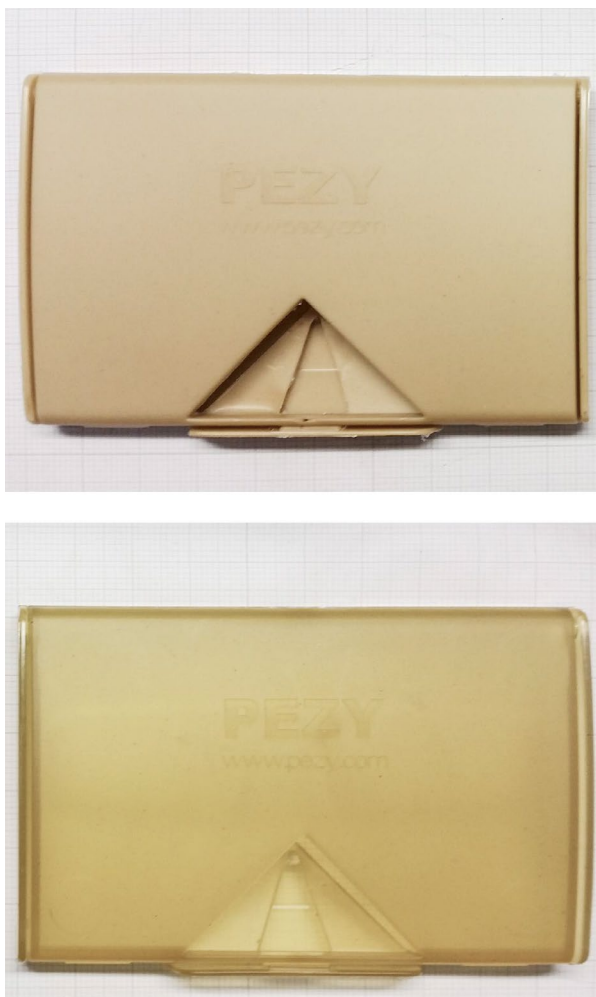
FIGURE 46 BUSINESS CARD HOLDERS INJECTED MOULDED BY PEZY GROUP. CARD HOLDERS WERE MADE WITH PHARIO BASED BIOPLASTIC FORMULATIONS WITH BIOMER-LIKE (UPPER), AND PLA-PHBV (LOWER) COMPOUNDS.
