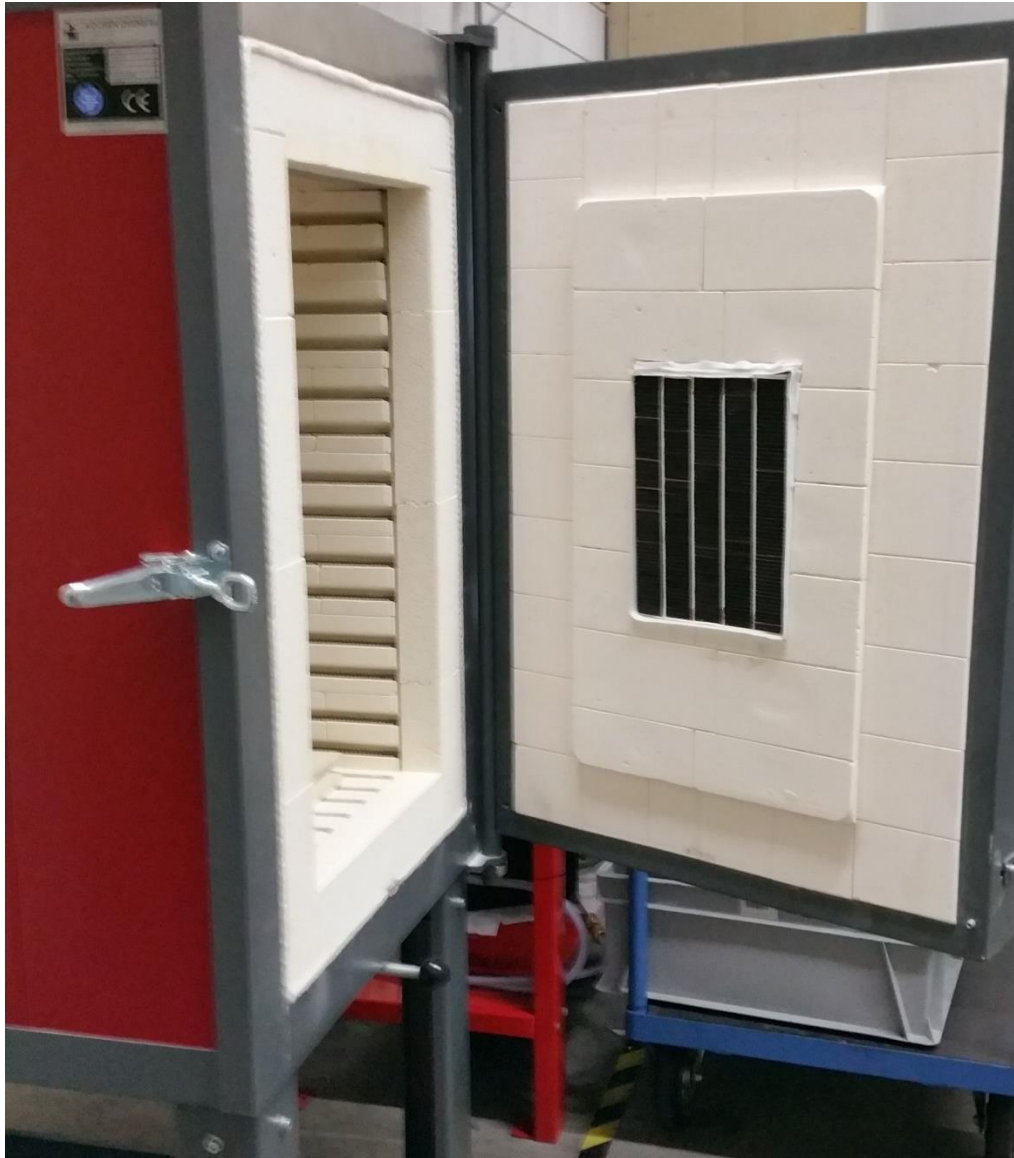
Figure 5: TEG panel in the door of a test furnace. In such furnaces duration tests of components were made prior to installation in the production environment.
