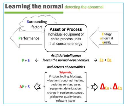
The energy amount **Ea** (and power quality **Eq**) vary most of the time normally with the performance **P** and surrounding factors **S** (for example a specific combination of Flow, pressure, temperature, quality, ambient temperature etc.).
