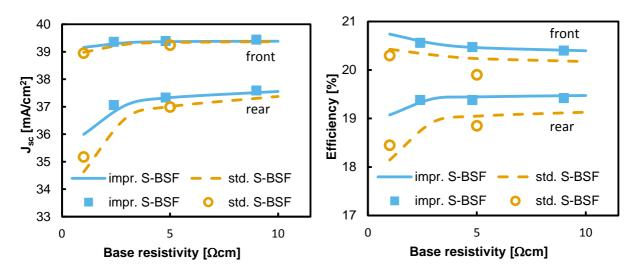
Looking at the efficiency, we see that both the front and rear efficiencies improve with the optimised BSF, but the effect is larger for the rear and most significant at low  $\rho$  base.
