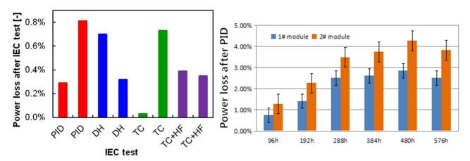
In conclusion, hot spot conditions are not likely to occur due to inhomogeneous rear irradiance. Yingli's double glass Panda modules are IEC qualified and pass all test with <1% power loss. Yingli's double glass Panda modules show less than 5% PID degradation even after prolonged exposure. The PID power loss also stabilises in contrast to shunt-PID in p-type modules where the power loss continues to >50%.
