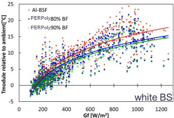
We also compared the same cell concepts in bifacial, glass-glass laminates. Again the laminate with the Al-BSF solar cell show the highest increase,  $+14^{\circ}$ C, with increasing front irradiance, and the laminate with the 90% bifaciality factor solar cell the lowest increase,  $+10^{\circ}$ C, above ambient.
