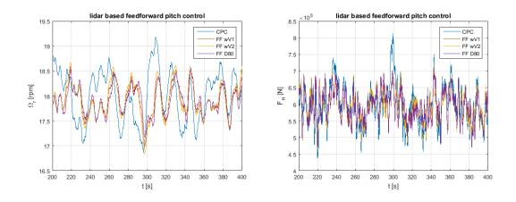
**Figure 14:** Wind turbine rotor speed and thrust response with LiDAR based feedforward collective pitch control featuring different weighting of the range gates (blue: no LiDAR, red: equal weighting, orange: increased weight towards the rotor, purple: single range gate at 80m)
