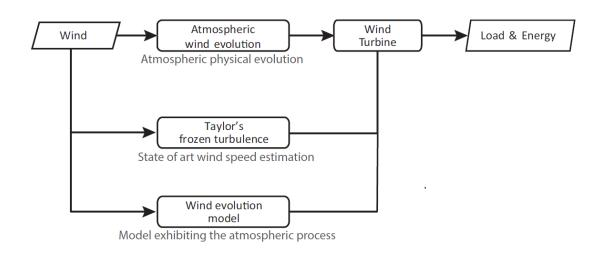
**Figure 13:** Process diagram illustrating the natural atmospheric process of wind evolution followed by two different approaches to resemble the modelling of this process, namely by Taylor's frozen turbulence assumption or using a wind evolution model. The latter being the objective of the PhD study, from [15].
