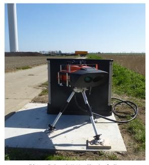
(a) Ground based LiDAR calibration facility
