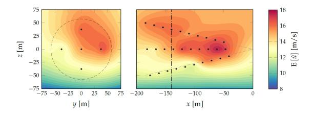
**Figure 15:** Stream wise mean velocity field based on one full cycle of measurements (1.25 s). The dots pinpoint the locations of the measurement points. Left: vertical plane parallel to rotor disc (140 m in front of the rotor). Right: vertical plane perpendicular to rotor disc (through rotor centre) [71].
