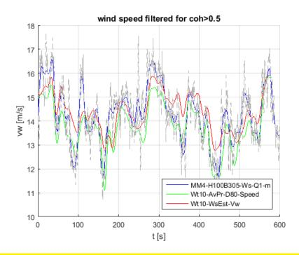
**Figure 10:** Time trace of the wind speed measured at the meteo mast (blue), the forward looking LiDAR at 80m range (green) and the estimated wind speed at the rotor plane (red)
