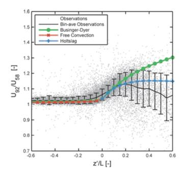
**Figure 4:** Wind shear ratio as a function of atmospheric stability (z'/L) according to observations and specific shear models (see legend). The solid thin line is the bin-averaged observations with error bars indicating one standard deviation within the bin [62].
