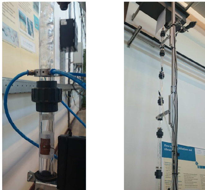
Figure 5.1 Left: Gas inlet and liquid inlet of the flow loop set up. The capacitance probes are mounted on the first segment. Right: top half of the flow loop connected downstream to the atmospheric air/water separator.
