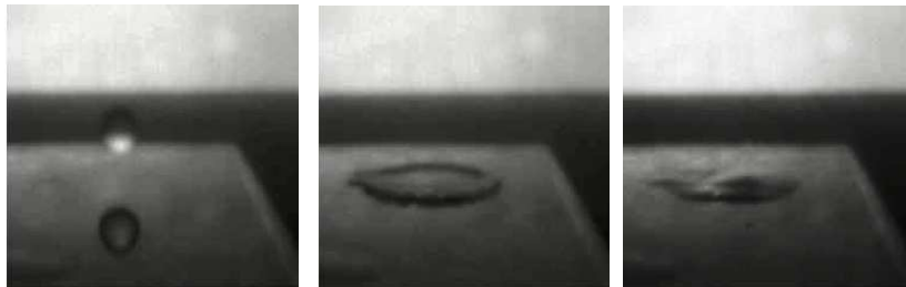
Figure 6.4 Droplet impinging on PMMA substrate (A). Left: just before impact, center: maximum wetting of the surface, right: maximum height of retracted droplet.
