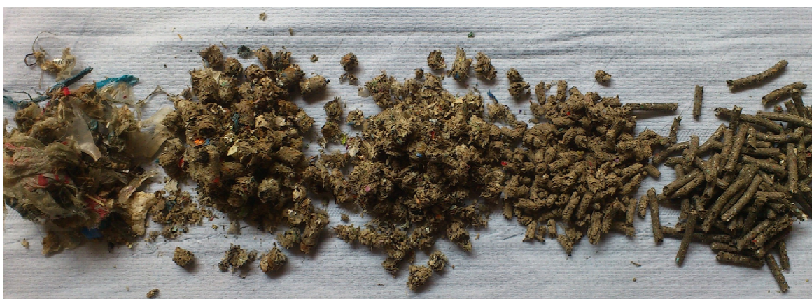
Paper rejects - Large pieces of metal and plastic removed. - 40-60% wt. moisture (wet basis) 1 x pelletization, 8 mm dye. 2 x pelletization, 8 mm dye. 6 x pelletization, 4 mm dye. Moisture ~ 35% wt. (wet). Air-dried to 5% wt. moisture. 1 x pelletization, 4 mm dye.
