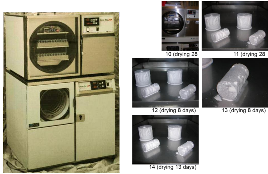
Figure 3-1 Freeze dryer and samples in freeze dryer.
