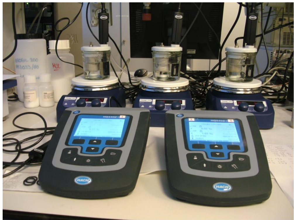
Figure 4-6: Setup to measure the salt dissolution rate of up to 4 samples in parallel (shown are three samples).
