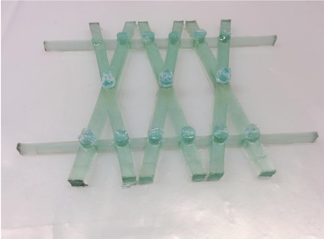
Figure 8.5: Picture of a grid just after infusion
