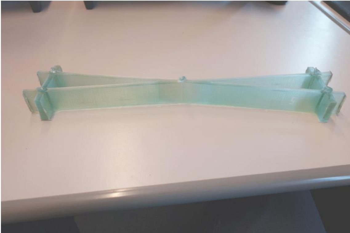
Figure 5.6: Picture showing the Final single helical node infusion sample
