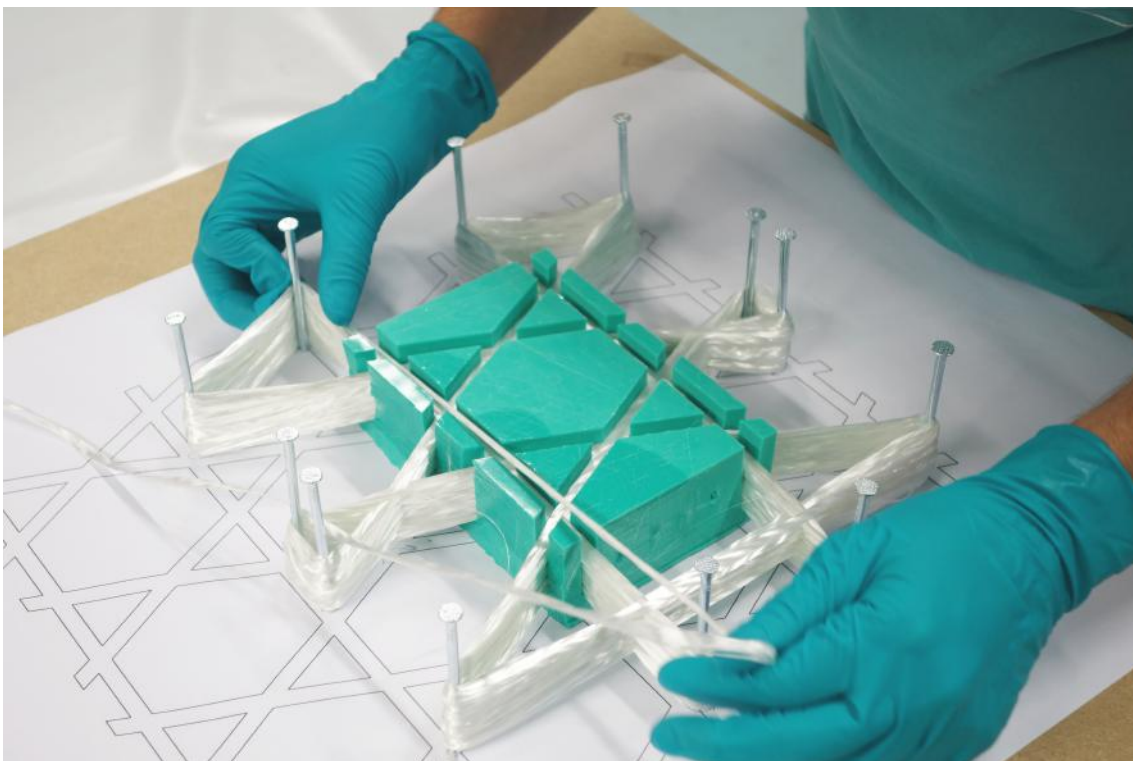
Figure 5.5: Picture showing the winding process of the high angle multiple helical node sample
