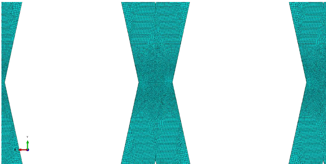
Figure 8.4: Close-up of the mesh at nodes
