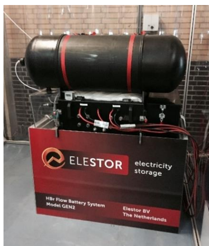
2 Elestor HBr flowbatterij systeem
