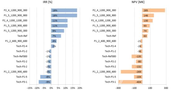
The graphs clearly show the good performance of the 1200 MW scenarios. The top 5 scenarios all have a 1200 MW interconnecting link. In addition, these top 5 scenarios are all based on DC technology. The difference between scenario P2\_4 and P1\_5 is the connection of the Dutch wind field with the interconnector, as also addressed in the introduction of this chapter. With these two scenarios with good performance and combination opportunities, we will further analyse the
