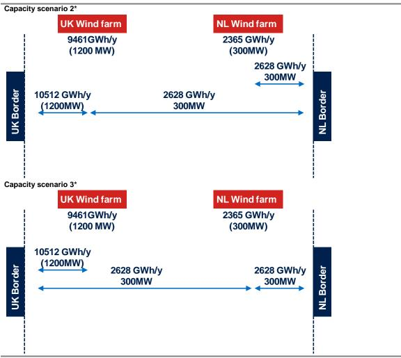
(\*) The capacities of the different scenarios shows the 300 MW interconnecting capacity. The analysis covers the 300 MW IL-scenarios as well as 1200 MW IL-scenarios.
