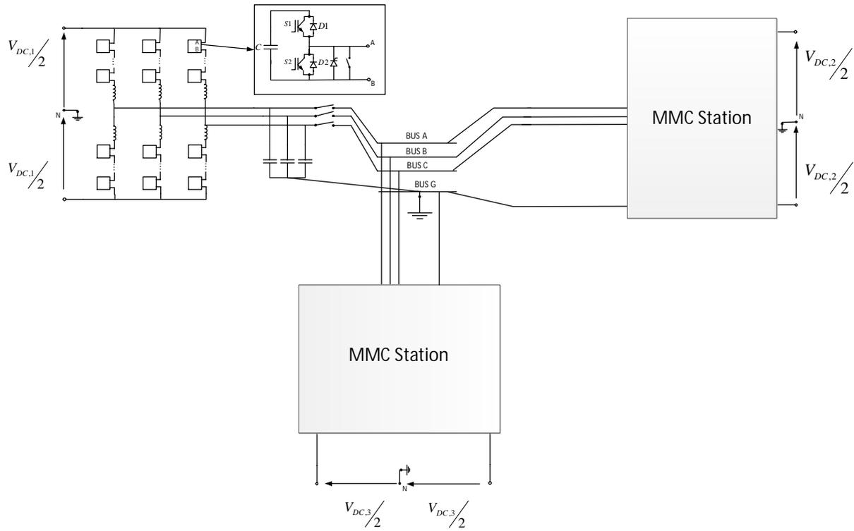
Figure 5-1. MMC-based DC hub.
