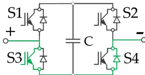
Figure 3-7: Current path through the H-bridge submodule.
