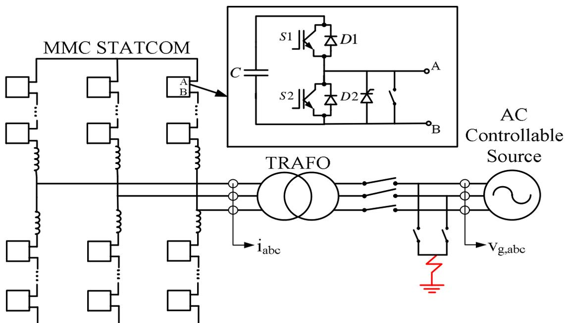
Figure 4-2: STATCOM Lab connection.
