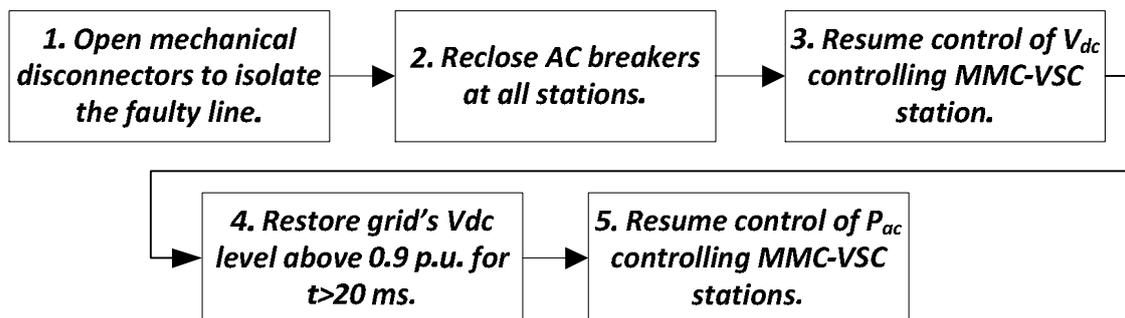
Figure 3-5. Framework for dc grid restoration.
