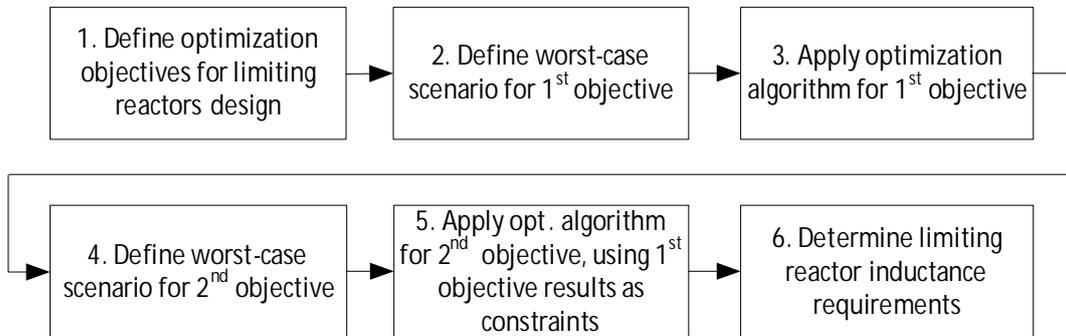
Figure 3-2. Methodology for the design of dc limiting reactors.
