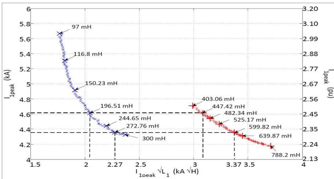
Figure 3-3. Relative cost, mass and peak dc current for optimized limiting reactor solutions at one converter stations (blue: solid-state breakers, red: hybrid breaker).
