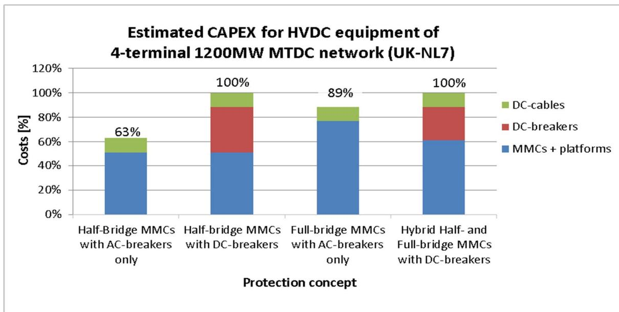
Figure 6-2: Estimated costs for HVDC components relative to DC-breaker solution
