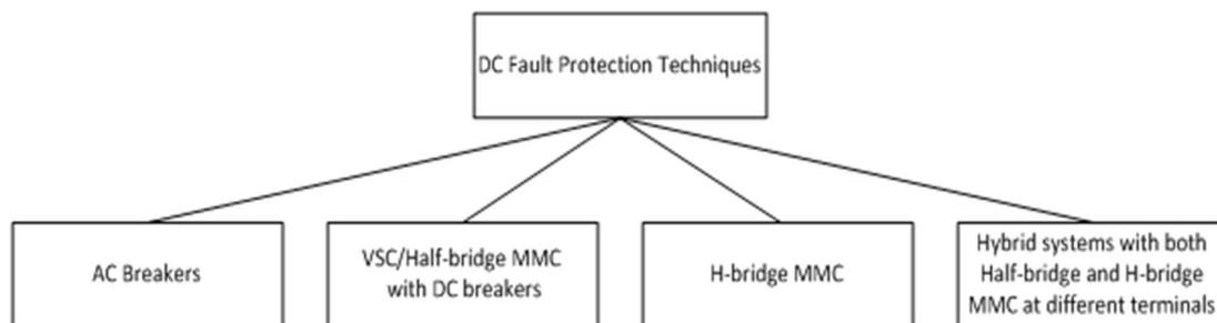
Figure 6-1: Different DC fault protection techniques.
