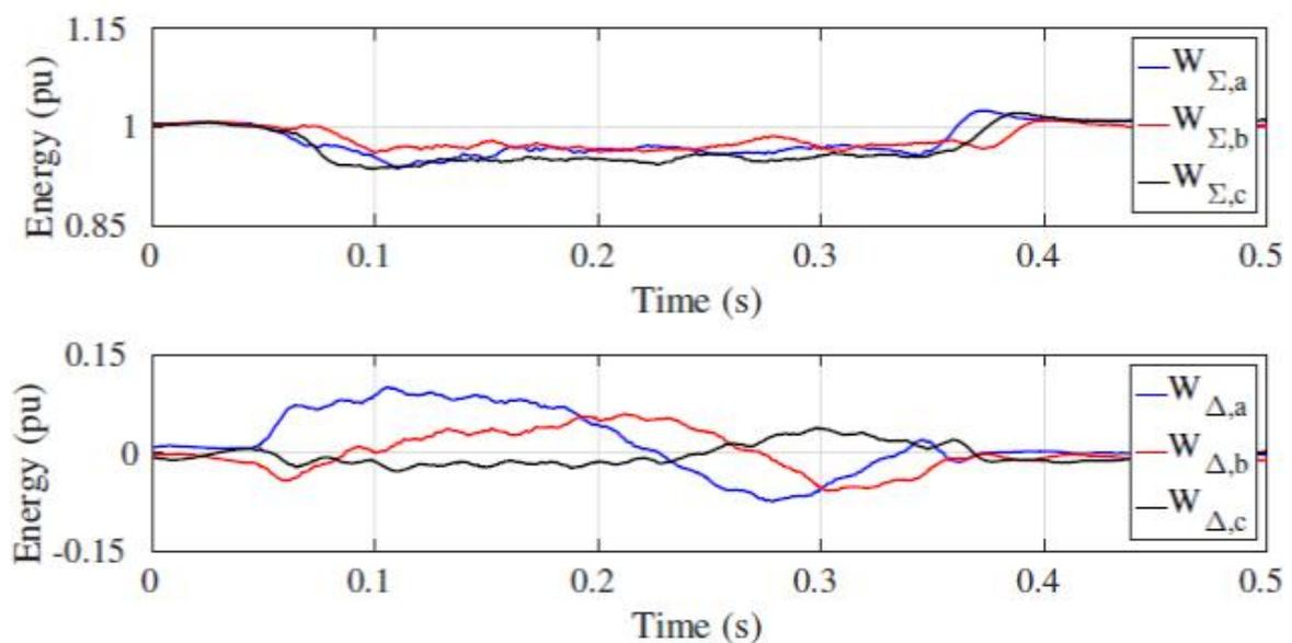
Figure 4-4:  $W_{\Sigma}$  and  $W_{\Delta}$  for experimental scenario with energy controllers.
