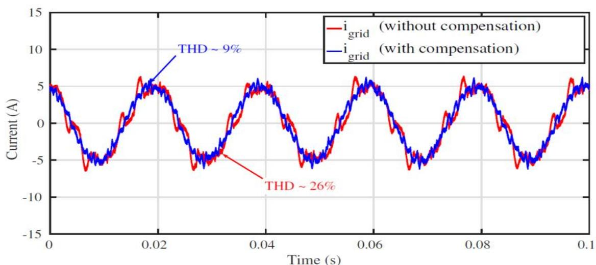
Figure 4-5: Grid currents before and after compensation.
