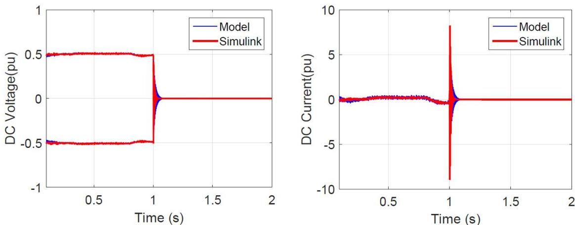
Figure 2-2. (a) Pole dc voltage and (b) Pole dc current at the output of an MMC attached to the dc faulty line.
