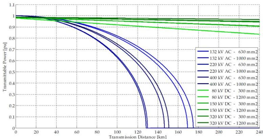
Figure 1-2: Maximum transferrable power as a function of transmission distance.
