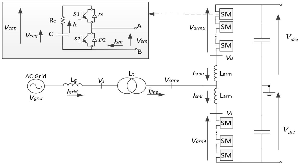
Figure 2-1. Model of a half-bridge MMC.
