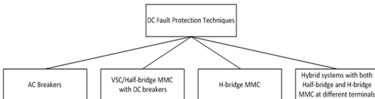
Figure 1-2: Different DC fault protection techniques.
