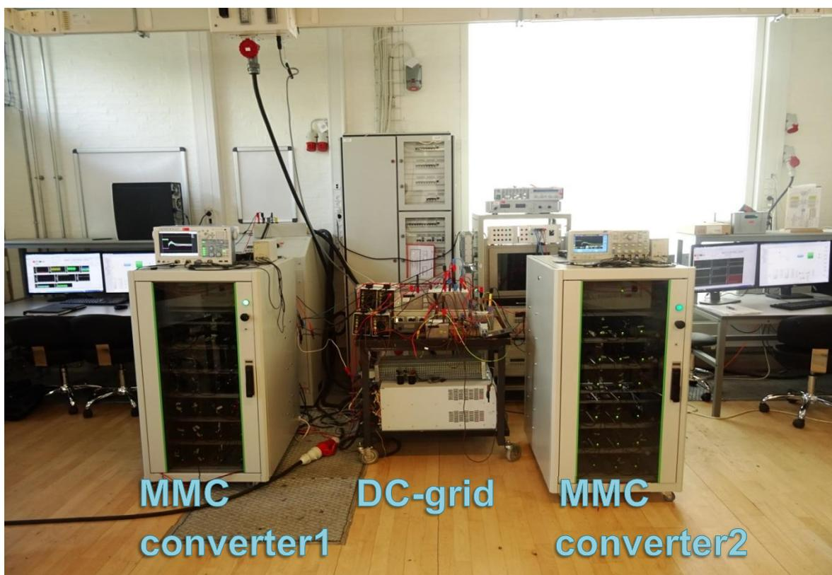
Figure 4-1: Laboratory set-up at Aalborg University applied for validation
