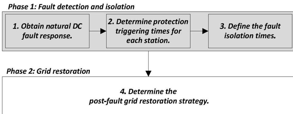
Figure 3-4. Methodology for dc fault ride-through studies.
