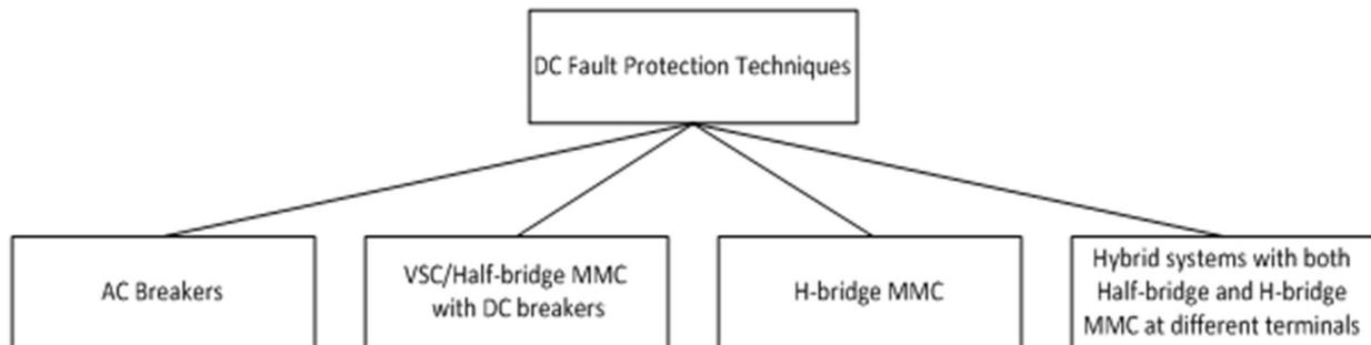
Figure 3-1: Different DC fault protection techniques.
