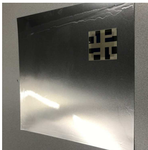
Figure 1 Example of a 6 inch stainless steel foil coated with an isolating barrier coating. Also presented is a 3 cm x 3 cm test structure for preparing devices on the foil with coating.
