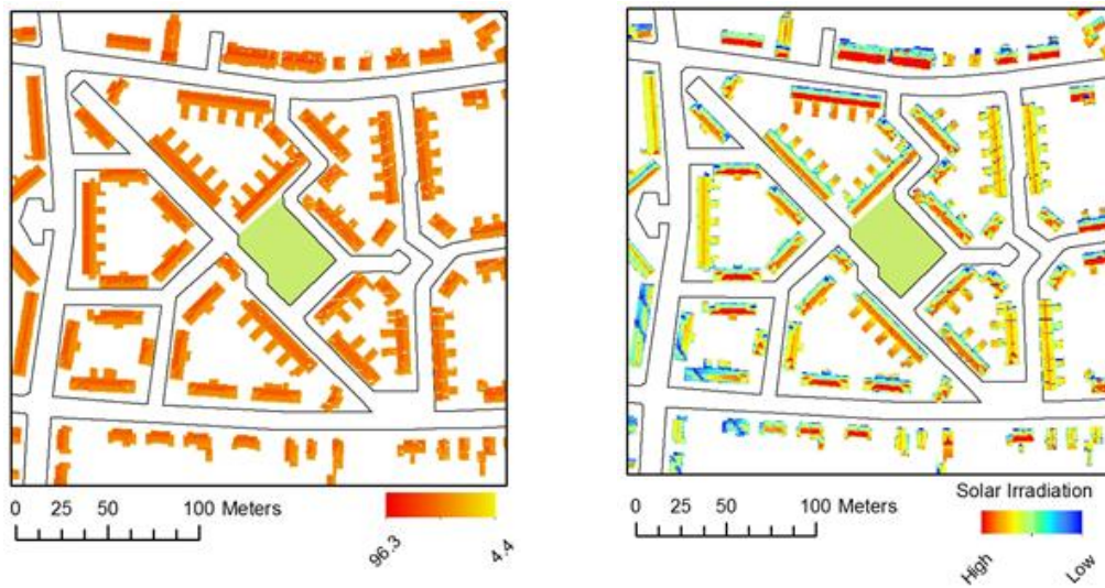
Figure 5: (Left) AHN height information derived for residential buildings. Height information is in meters. (Right) Solar Irradiation image derived for building by running the Solar Radiation tool. South facing slopes are seen to receive greater irradiation
