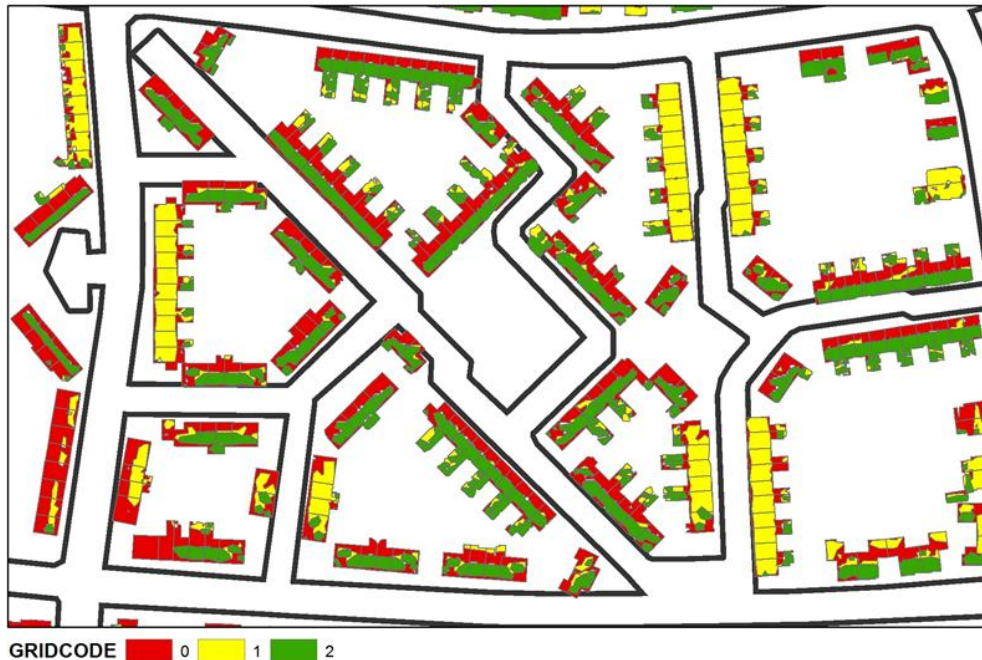
Figure 9: Final output showing the geographic potential of Apeldoorn city using Method 1. Gridcode 0 shows unfeasible areas, 1 represents partially suitable area and 2 shows best suits areas for the deployment of PV.
