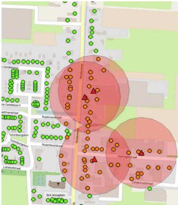
**Figure 10: Overlapping electrical supply areas and address outside electrical supply area**
