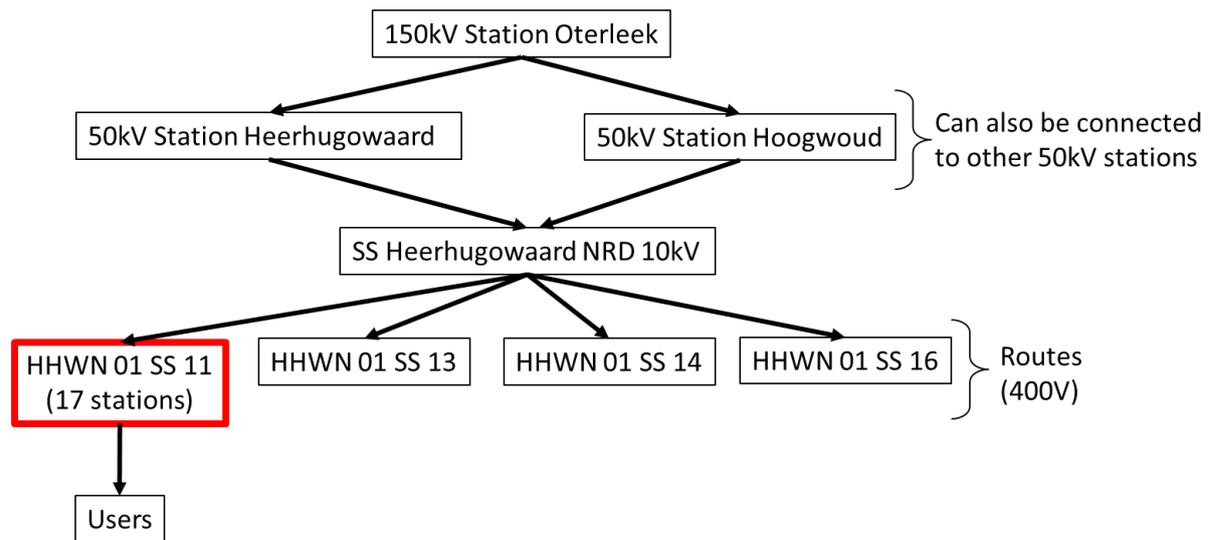
**Figure 9: Hierarchical structure of the electrical grid in the area of Heerhugowaard**
